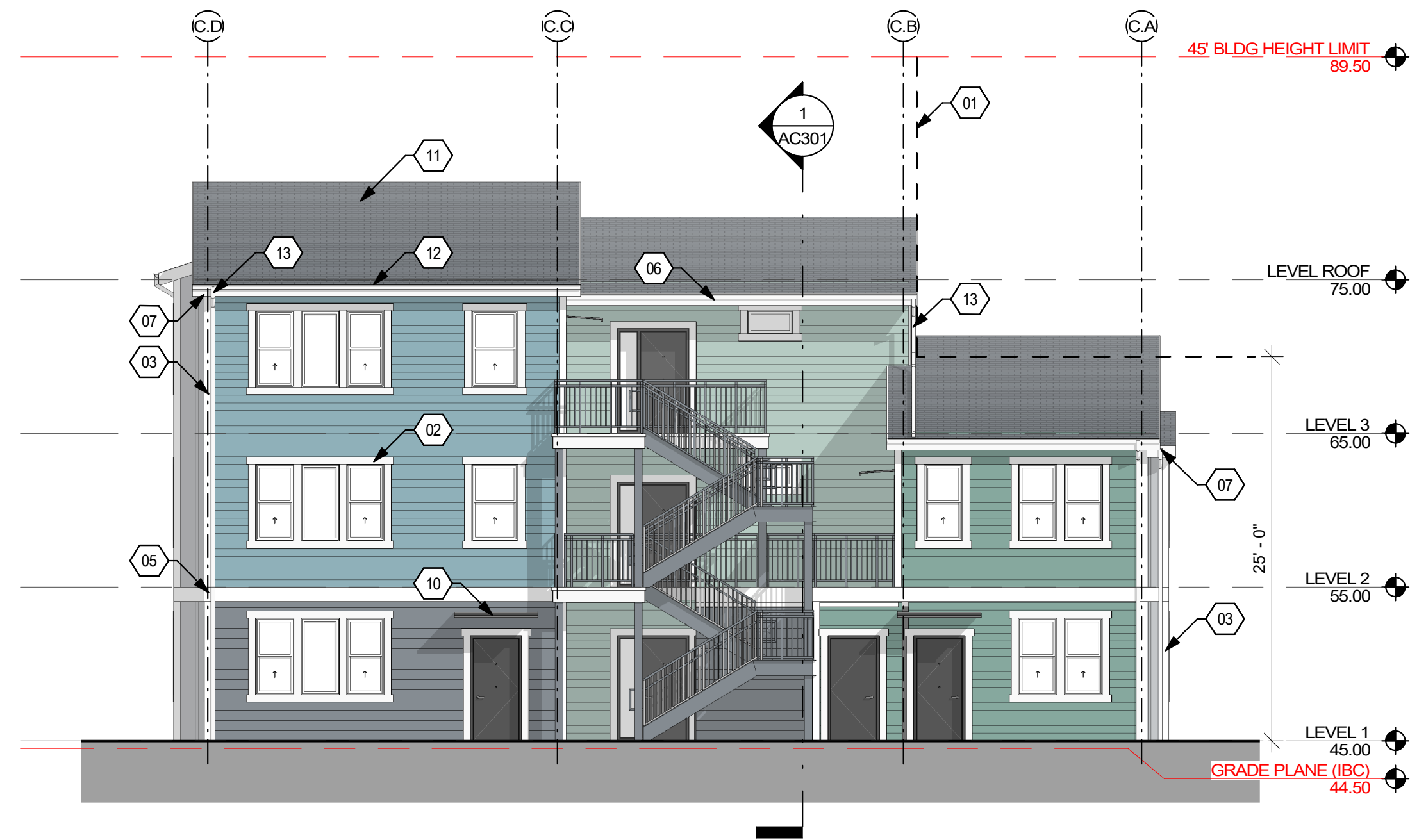
1 BLDG C - NORTH ELEVATION SCALE: 1/8" = 1'-0"
