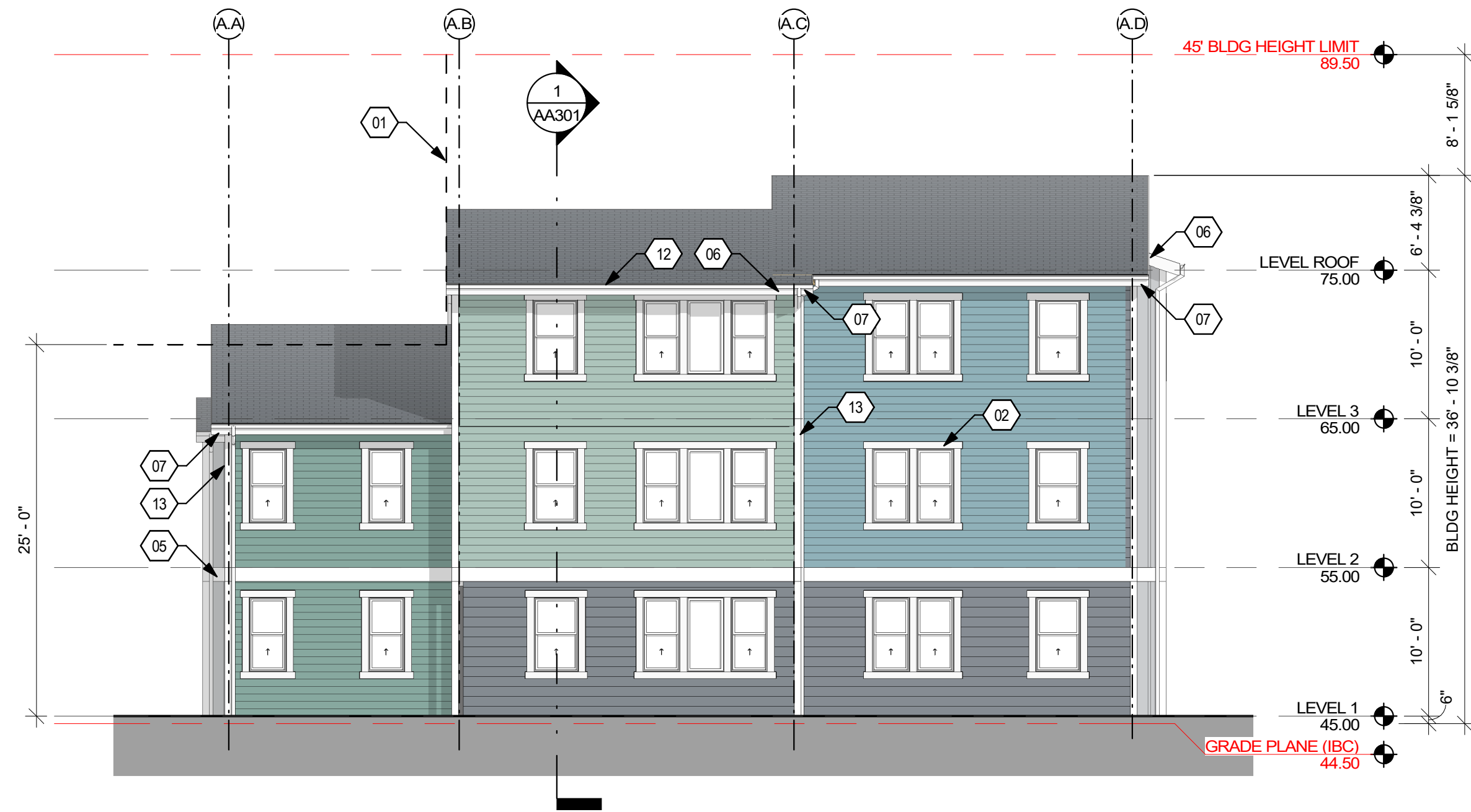
2 BLDG A - SOUTH ELEVATION SCALE: 1/8" = 1'-0"
