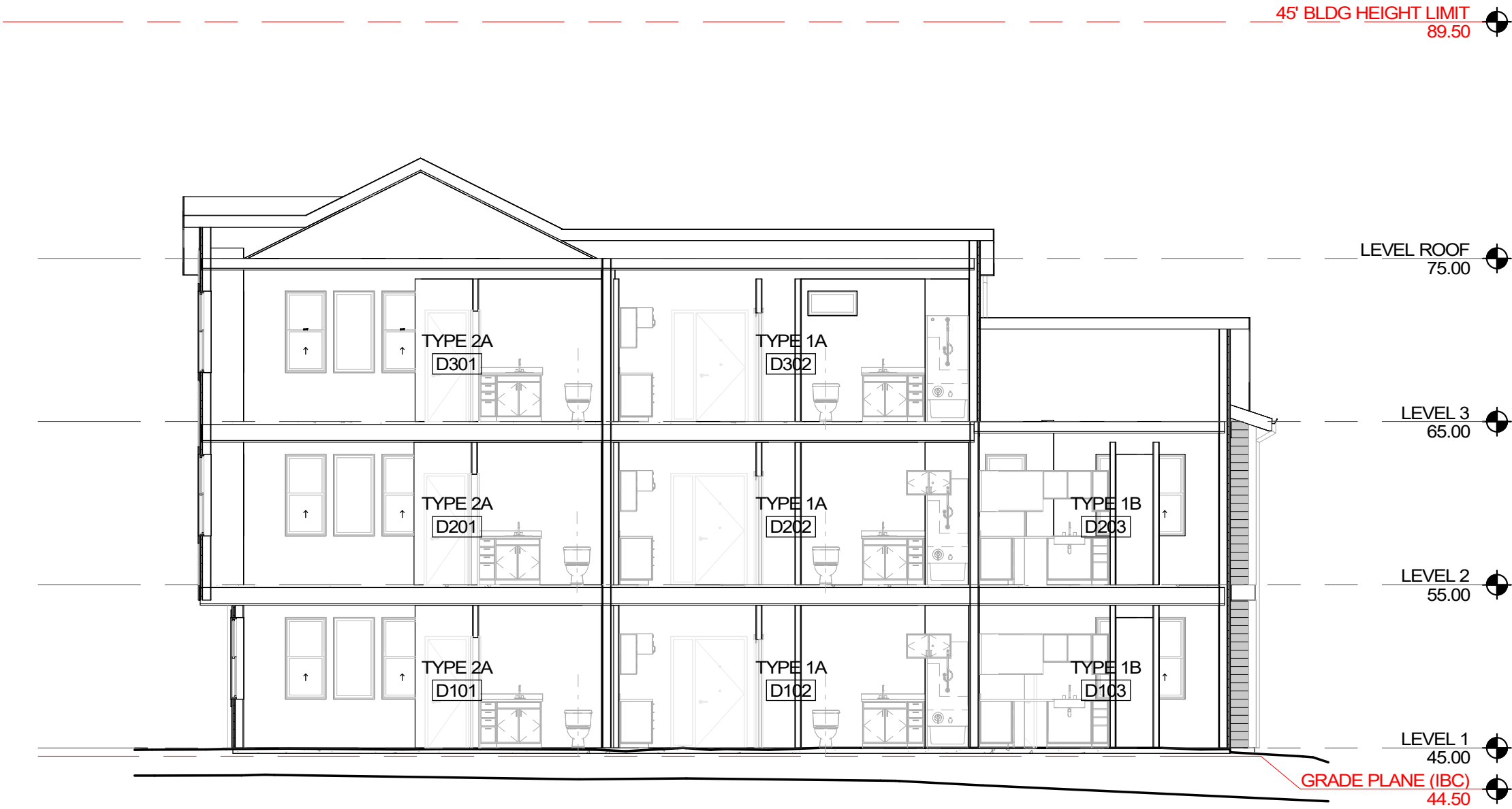
1 BLDG D EAST-WEST SECTION SCALE: 1/8" = 1'-0"
