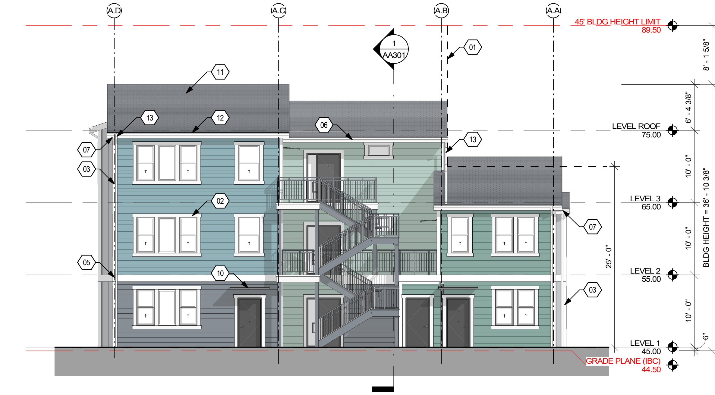
1 BLDG A - NORTH ELEVATION SCALE: 1/8" = 1'-0"
